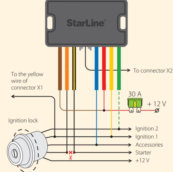
Set X2:6 blue wire as Starter protection and X2:15 orange wire as Engine start: ACC in StarLine Master configuration program.
